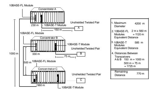
Figure 2-7. Sample Configuration Distance Calculation
